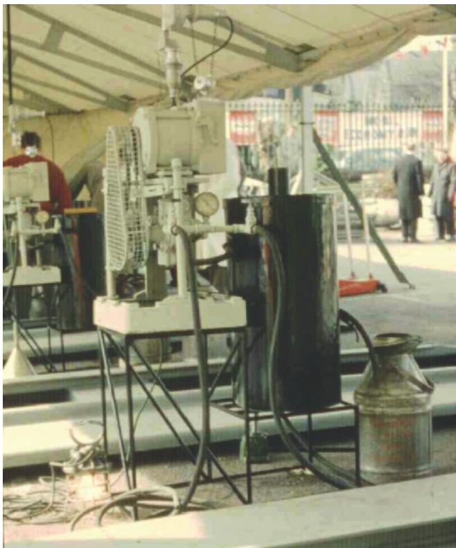
Powerful suction pump and condenser. We had to be sure to select the car's supply pipe rather than the return to suck from
